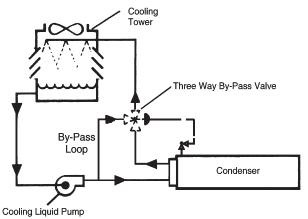
The aim is to maintain a stable discharge pressure as low as possible, but at least 5.0 bar above suction pressure. This can be done at a fixed value above the highest expected suction pressure, or by also measuring suction pressure and using differential control. In either case condenser cooling liquid flow and temperature limits must also be observed.
